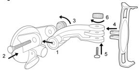
Assemble the cradle as shown in the illustration. No tools are needed for this.
